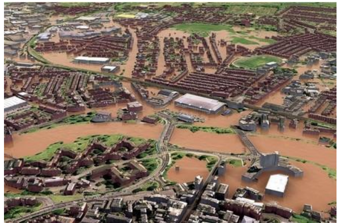
3D modelling of 1% flood event in central Exeter
